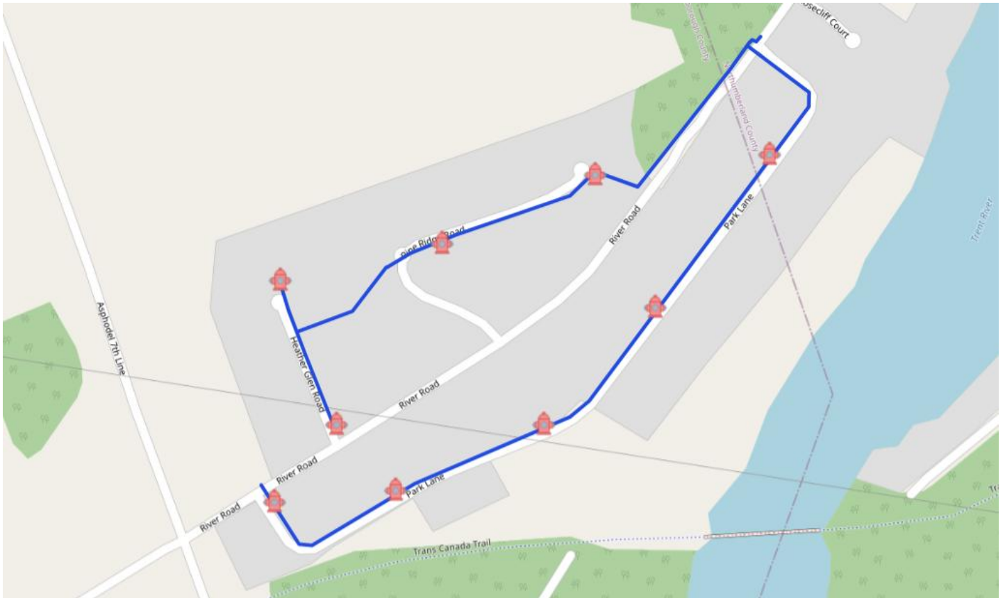
Figure 80 Trentview Estates Water Distribution and Hydrant Network
