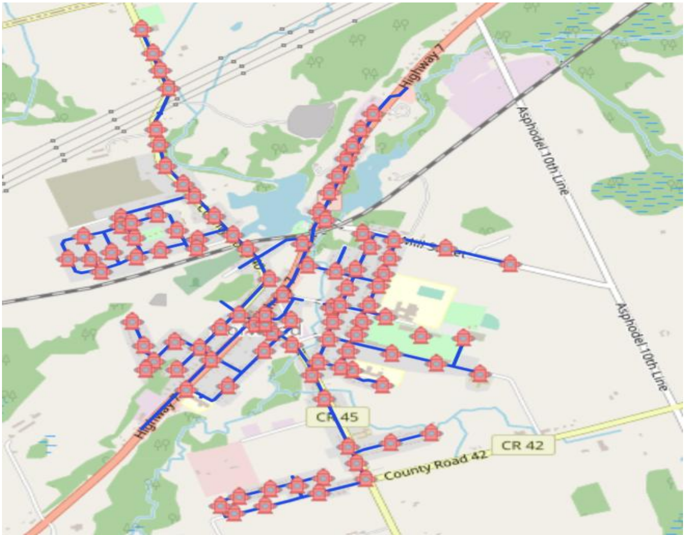
Figure 79 Norwood Water Distribution and Hydrant Network
